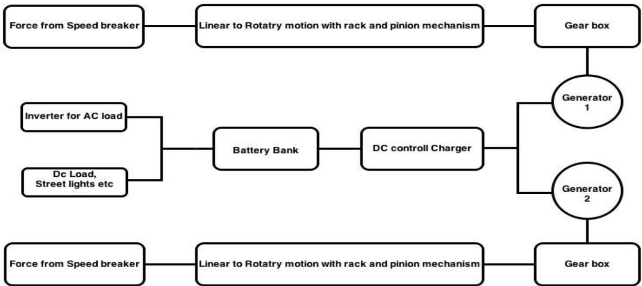
Fig. 5. Block diagram of PGS
