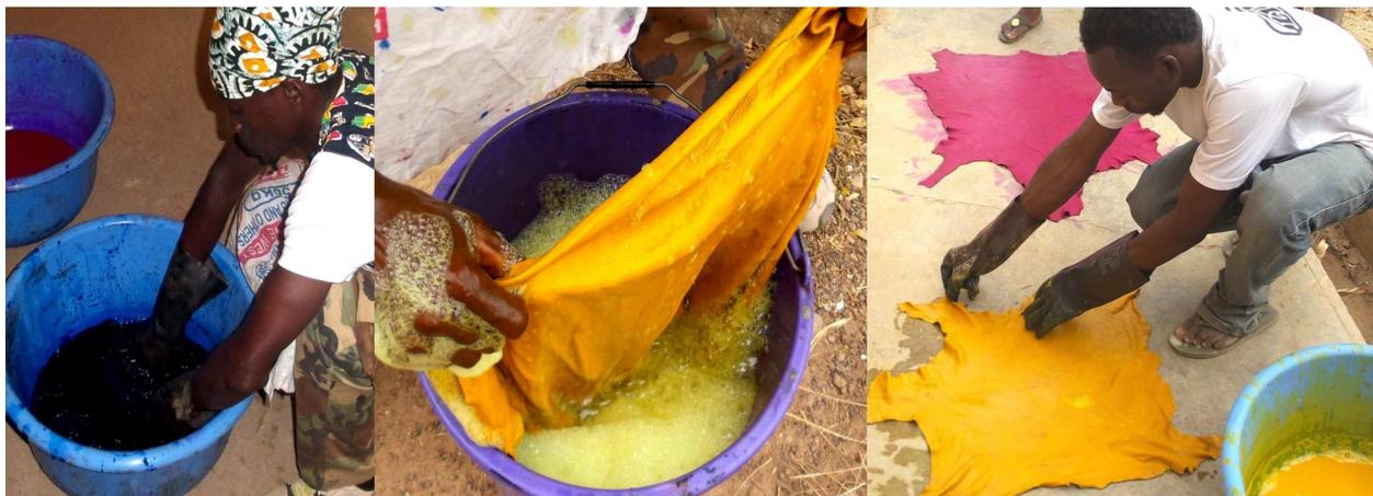
*Fig. 3. Dyeing of leather (left), Washing of leather (middle) and Drying of leather (right)*
