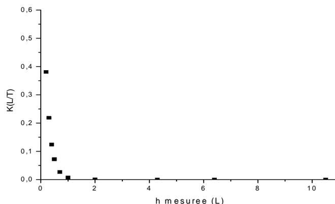
Figure 6. Measured hydraulic conductivity
