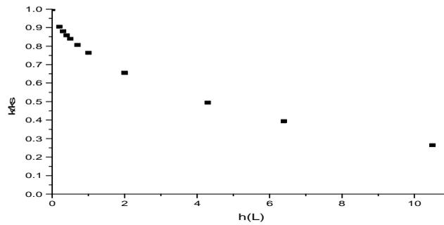
Figure 5. Calculated relative hydraulic conductivity ( $k/k_s$ )
