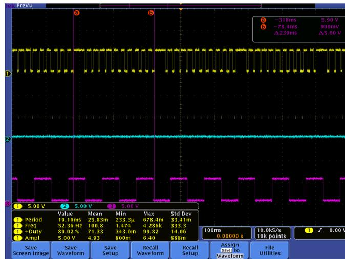
Fig.8 Response of proximity sensor on detection of a tooth of an encoder disc
