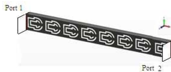
Figure 8: A periodic network formed by 8 cells in the shape of dome.
