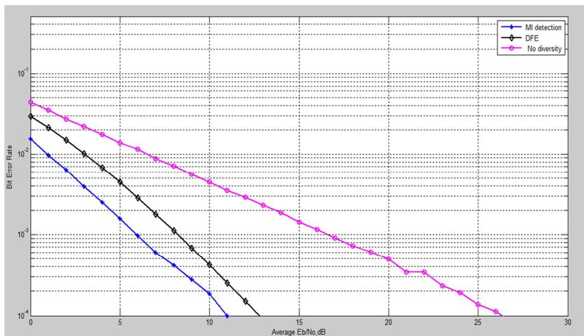
Fig. 4. BER of SFBC-OFDM system using 2Tx and 2Rx for Nakagami MIMO fading channel for  $m=4$ , 16QAM with frequency domain equalization
