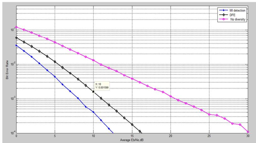
Fig. 3. BER of SFBC-OFDM system using 2Tx and 2Rx for Nakagami MIMO fading channel for  $m=2$ , 16QAM with frequency domain equalization
