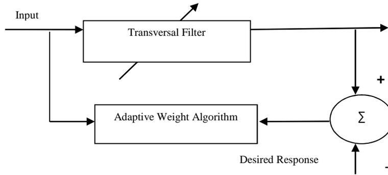
Fig. 2. Functional Block Diagram of DEF
