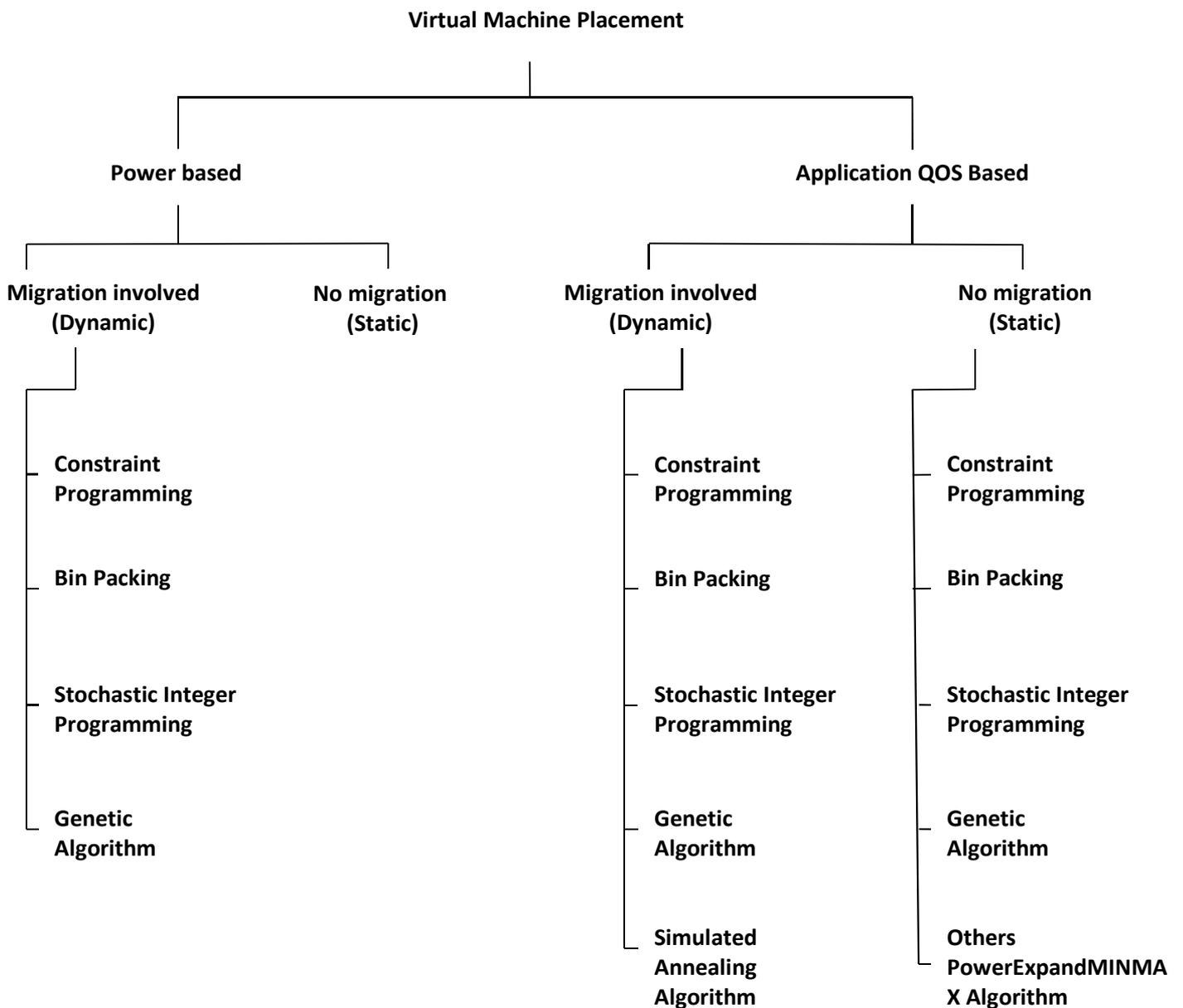
Fig. 2. Classification of VM Placement Algorithms
