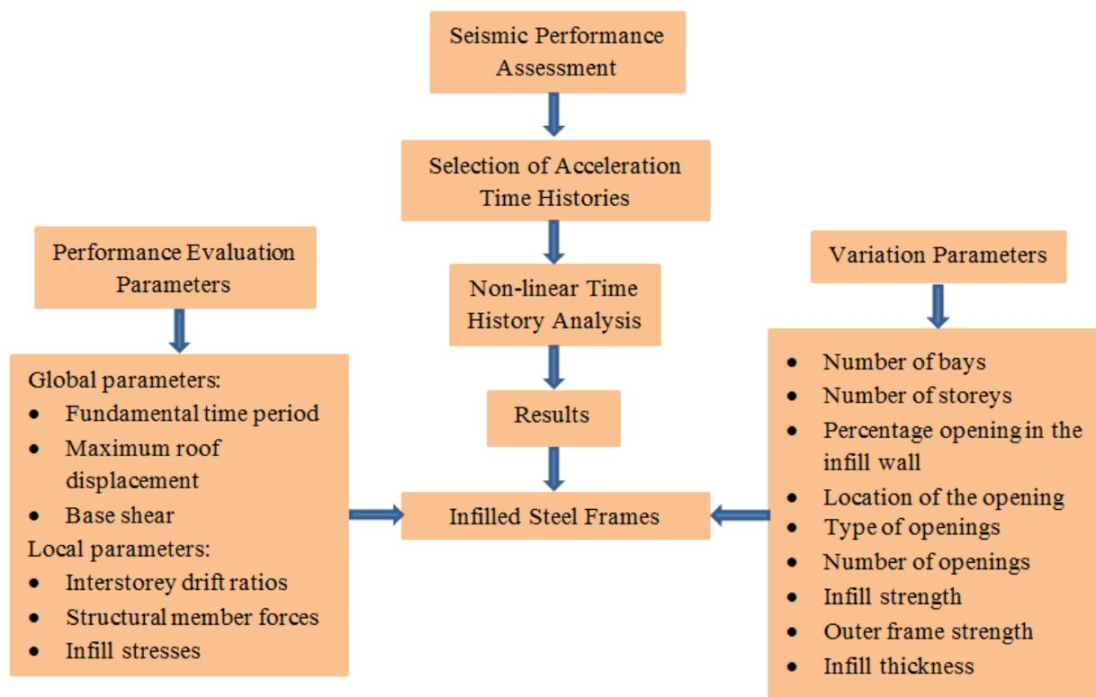
Figure 1: Seismic Performance Assessment (Flow Chart)
