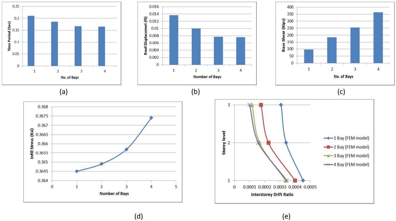
Figure 3: Effect of variation of number of bays on (a) Structural Period (b) Maximum roof displacement (c) Base shear (d) Infill stresses (e) Interstorey drift ratios
