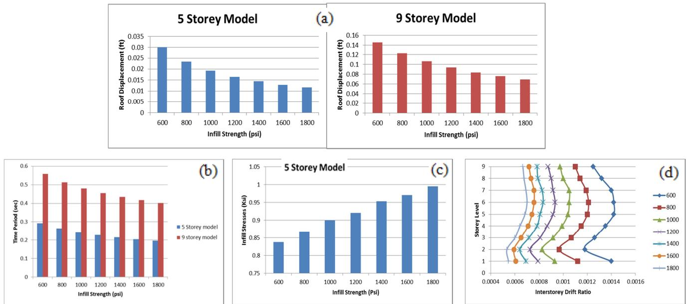
Figure 14: Effect of Variation of Infill Strength on (a) Maximum roof displacement (b) Structural Period (c) Infill stresses (d) Interstorey drift ratios
