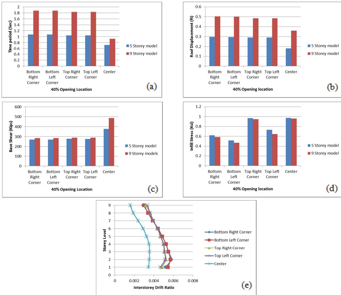
Figure 9: Effect of Different opening locations on (a) Structural Period (b) Maximum roof displacement (c) Base shear (d) Infill stresses (e) Interstorey drift ratios
