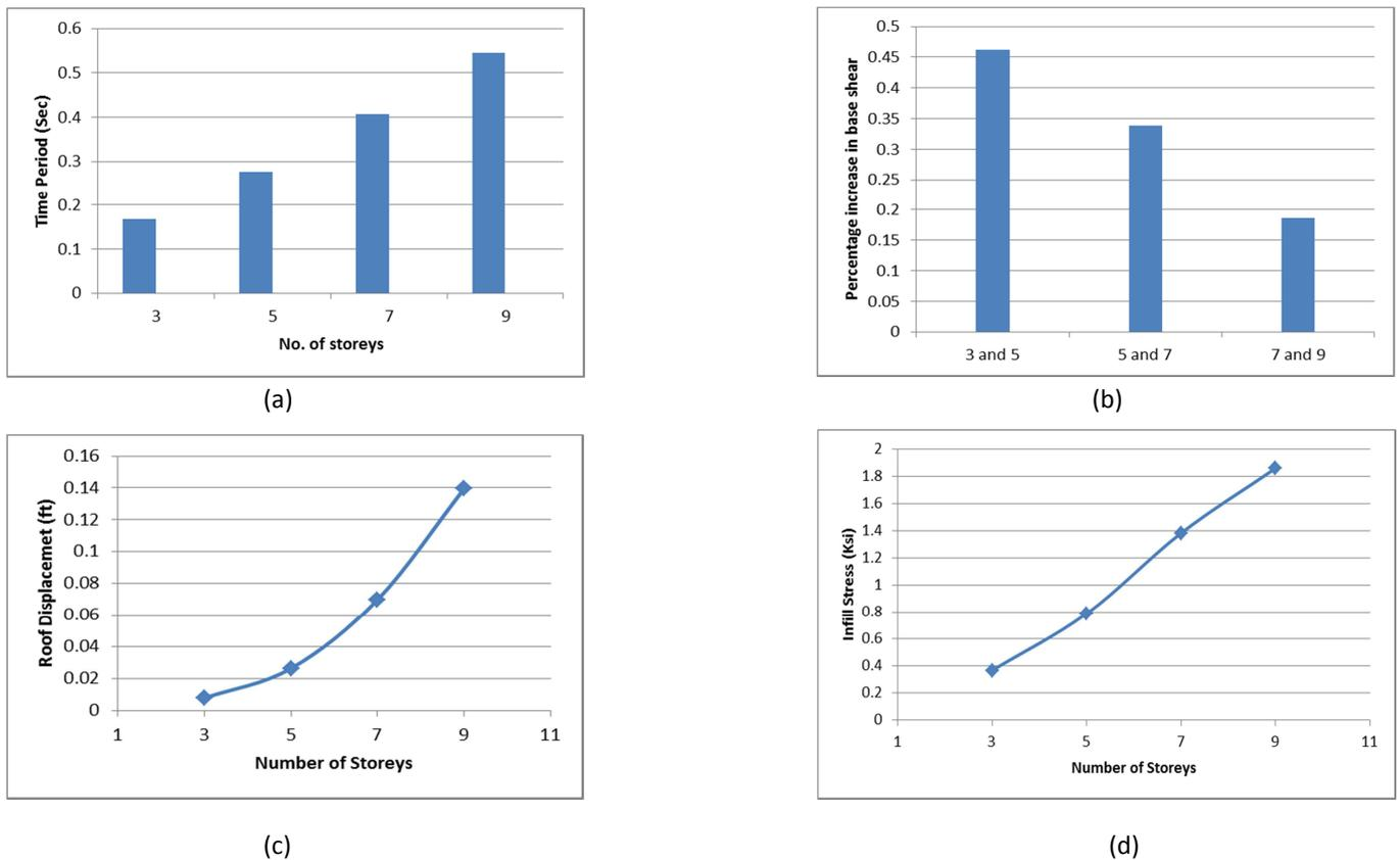
Figure 4: Effect of variation of number of storeys on (a) Structural Period (b) Base shear (c) Maximum roof displacement (d) Infill stresses
