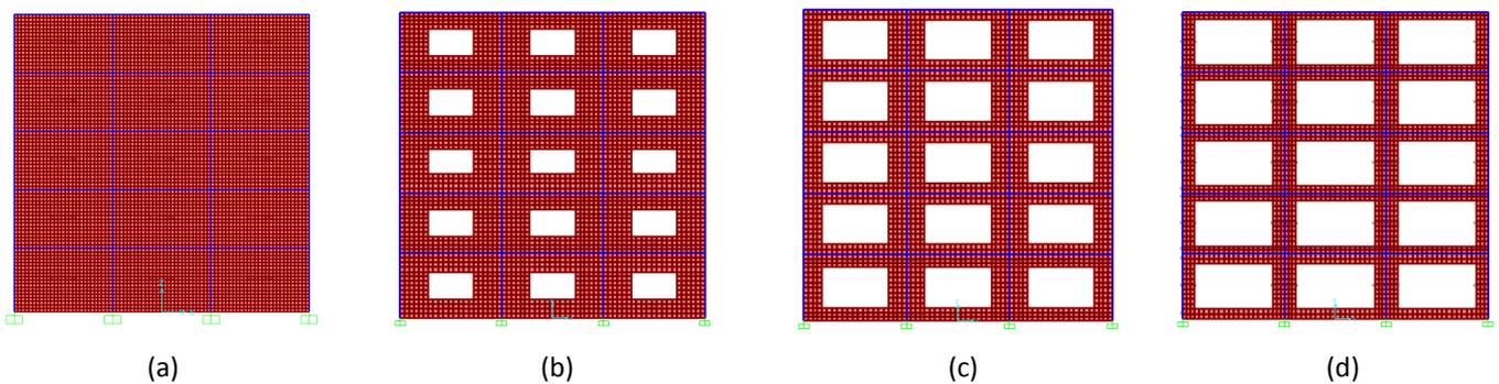
**Figure 5: 5 Storey model with different percentages of openings in the infill (a) Fully infilled (0% Opening) (b) 20% Opening (c) 40% Opening (d) 60% Opening**
