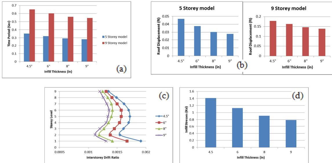
**Figure 15: Effect of Variation of Infill thickness on (a) Structural Period (b) Maximum roof displacement (c) Interstorey drift ratios (d) Infill stresses**
