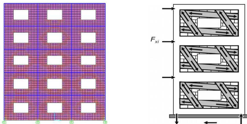
Figure 7: Compression stress path around an opening in comparison with FEMA 356
