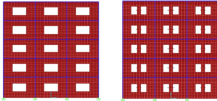
Figure 12: 20% single and dual opening for 5 storey steel infilled frame
