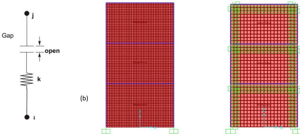
Figure 2: (a) Gap element (CSI Reference Manual SAP2000) (b) FEM Model with very fine meshing (c) FEM Model with Gap elements
