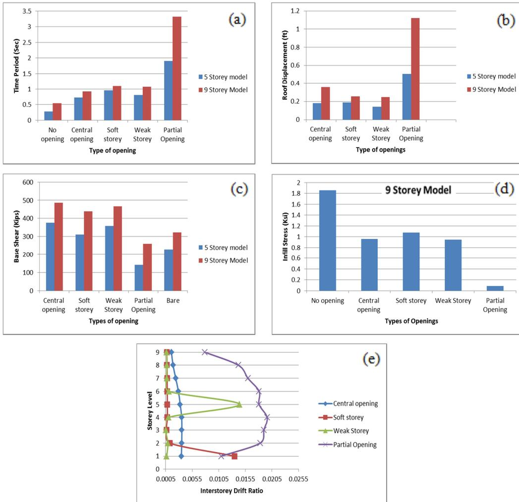
Figure 11: Effect of Different types of opening on (a) Structural Period (b) Maximum roof displacement (c) Base shear (d) Infill stresses (e) Interstorey drift ratios
