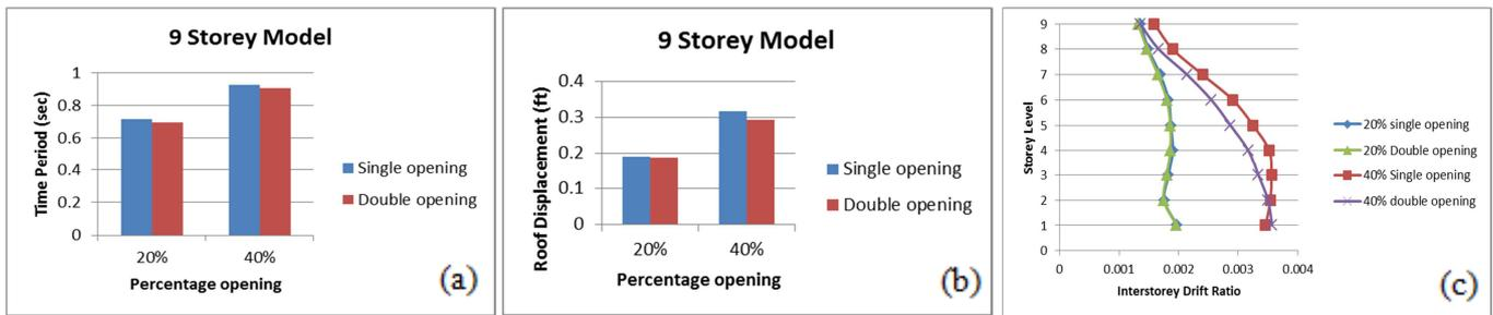
Figure 13: Effect of number of openings on (a) Structural Period (b) Maximum roof (c) Interstorey drift ratios
