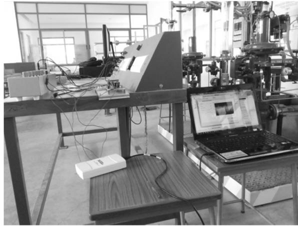
**Fig. 2.** The experimental setup of pneumatic actuator fault diagnosis
