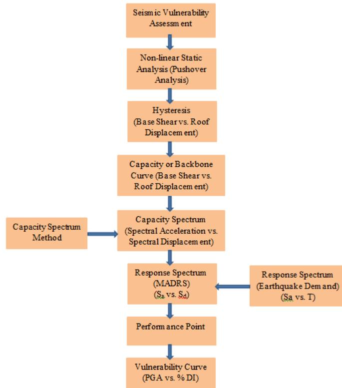
Figure 1: Seismic Vulnerability Assessment (Flow Chart)
