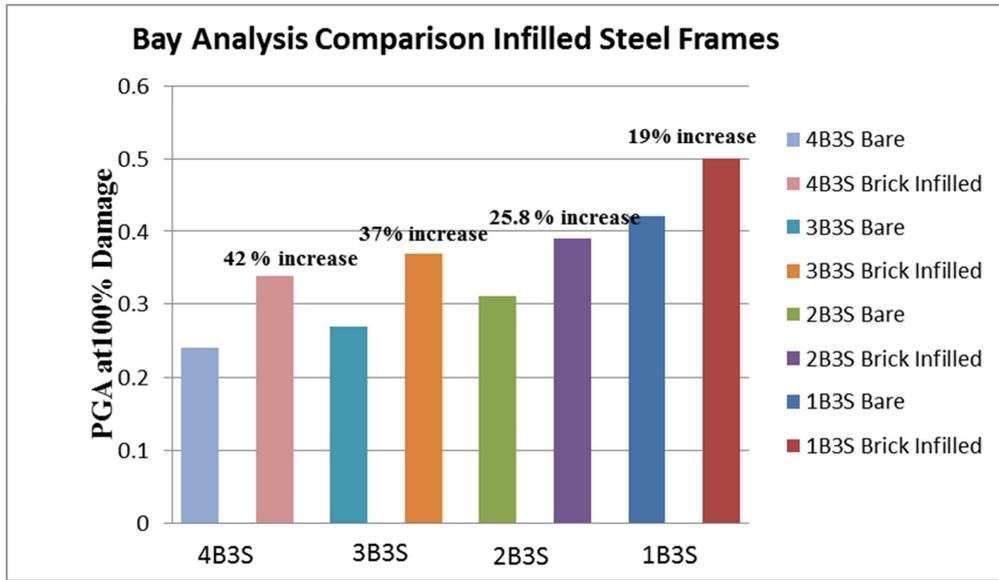
Figure 9: Comparison of PGA at 100% damage of Brick Infilled Steel frames with variation of number of bays.
