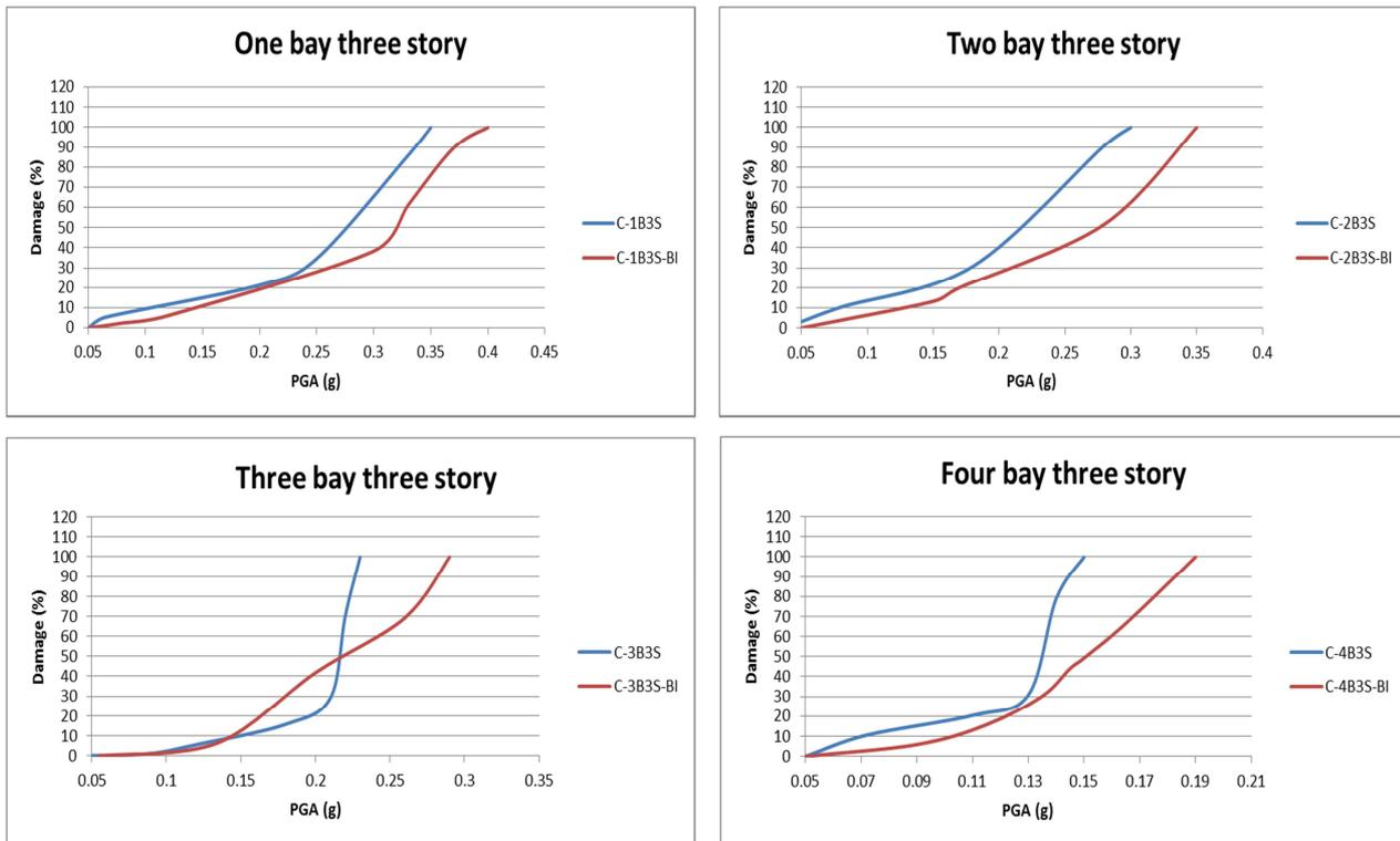
Figure-8: Vulnerability curves for bare and brick infilled (BI) RC frames
