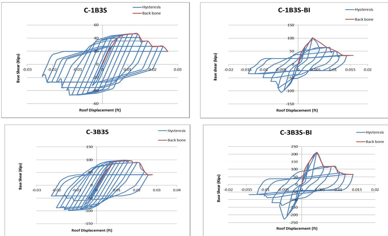
Figure-6: Hysteresis loops for 1 bay 3 storey (1B3S) and 3 bay 3 storey (3B3S) bare and brick infilled (BI) RC frames
