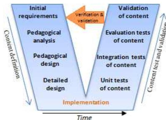
Fig. 5. Life cycle of collaborative design process
