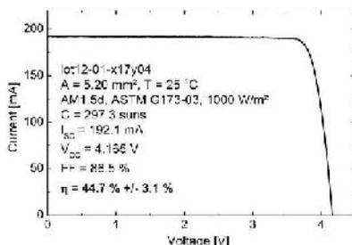
**Figure 5: Output response of a single solar cell.**
