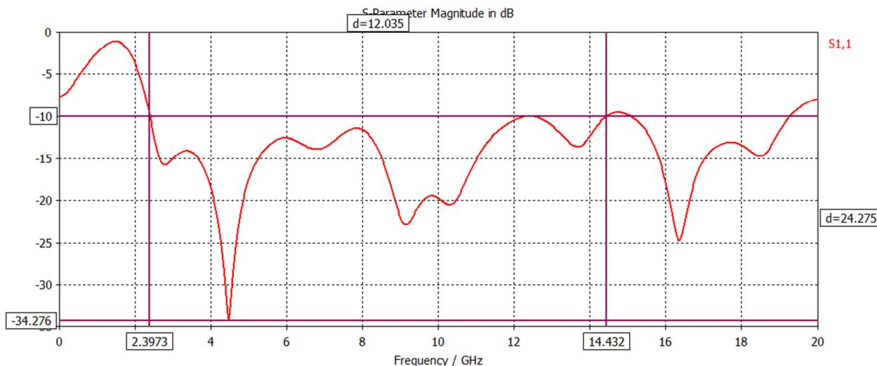
Fig. 3. Simulated  $S_{11}$  of proposed UWB antenna over free space
