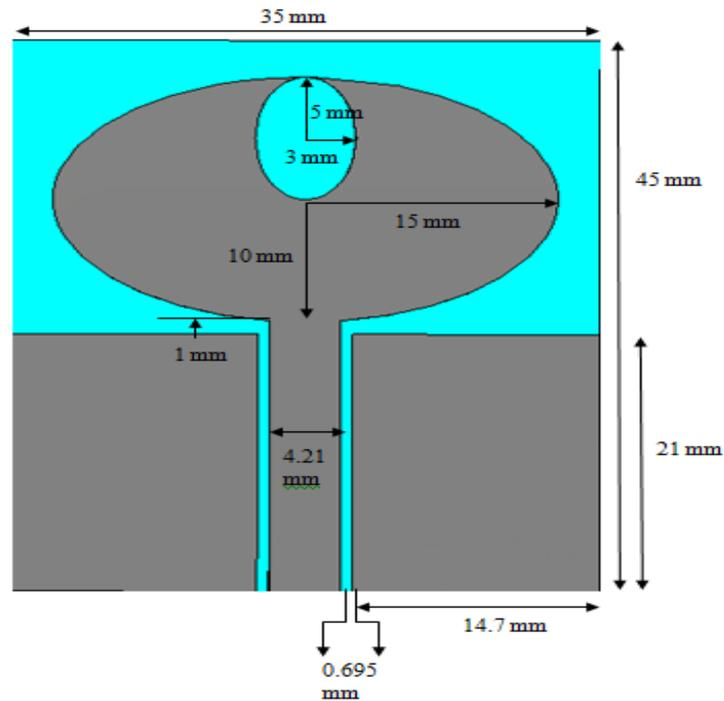
Fig. 1. Top view of designed Elliptical Patch UWB Antenna
