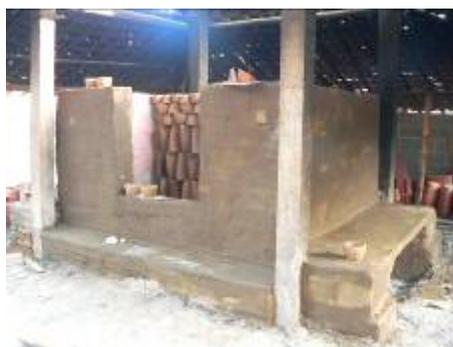
**Figure 13. Open vessel furnace with firewoods**
