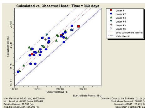
Fig 2. Head calibration for unlined canal
