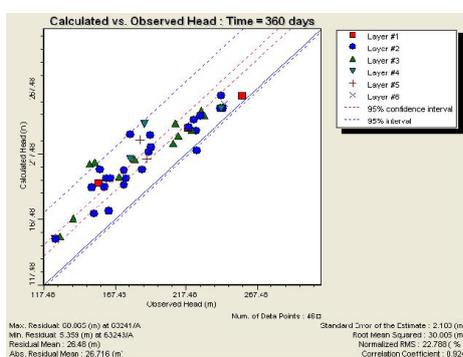
Fig 2. Head calibration for lined canal
