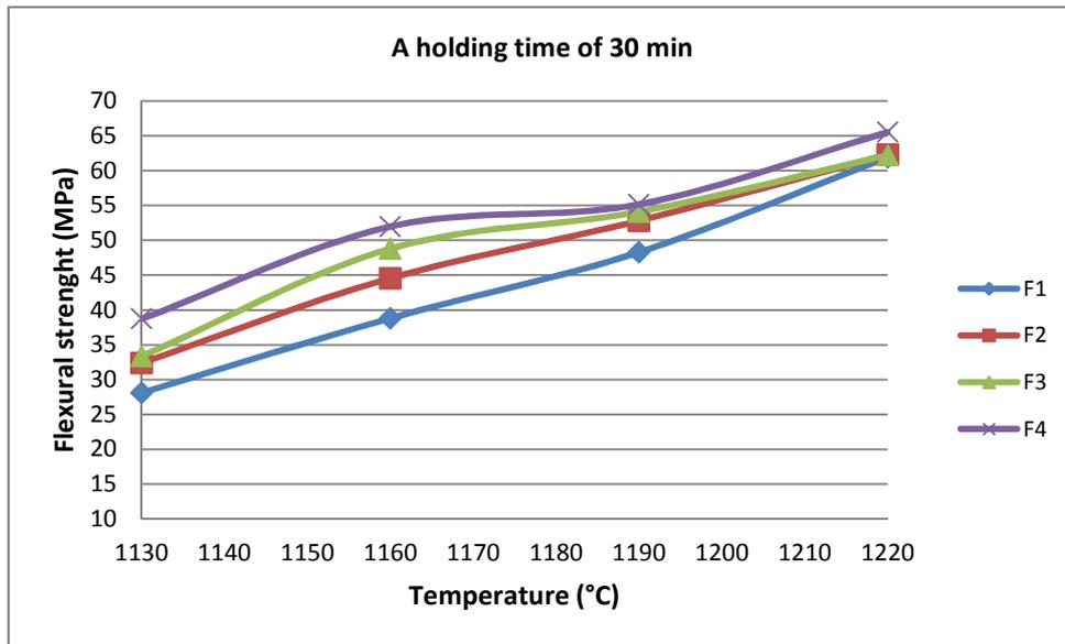
**Fig. 7.** The evolution of flexural strength of the four formulas according to the temperature at holding time equal to 30 min
