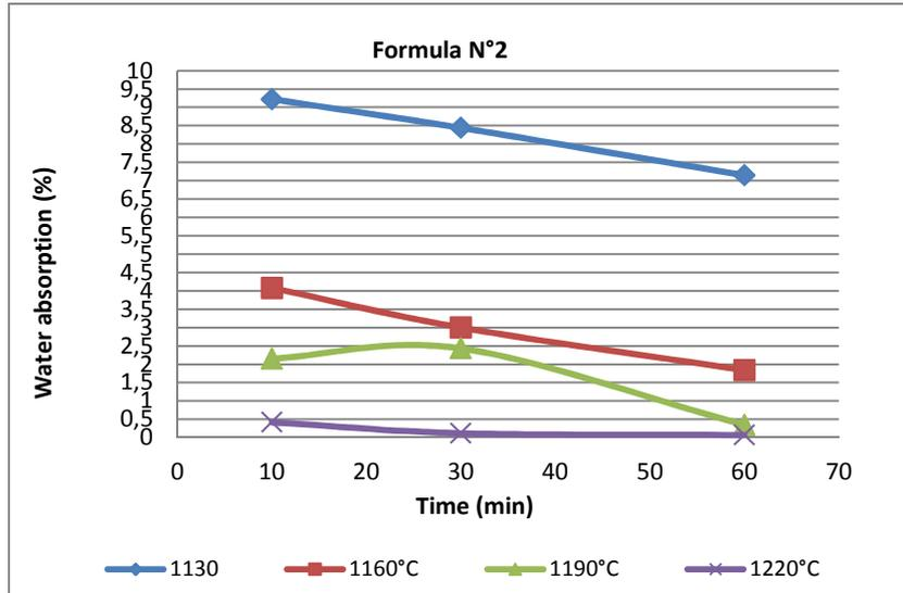
Fig. 2. Evolution of the water absorption of the formula n°2 according to the holding time at various temperatures of firing
