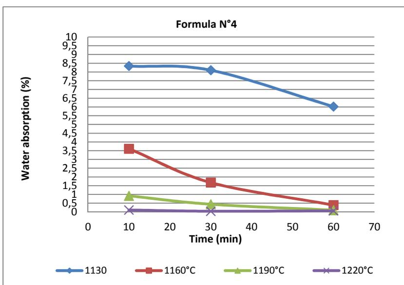
Fig. 4. Evolution of the water absorption of the formula n°4 according to the holding time at various temperatures of firing
