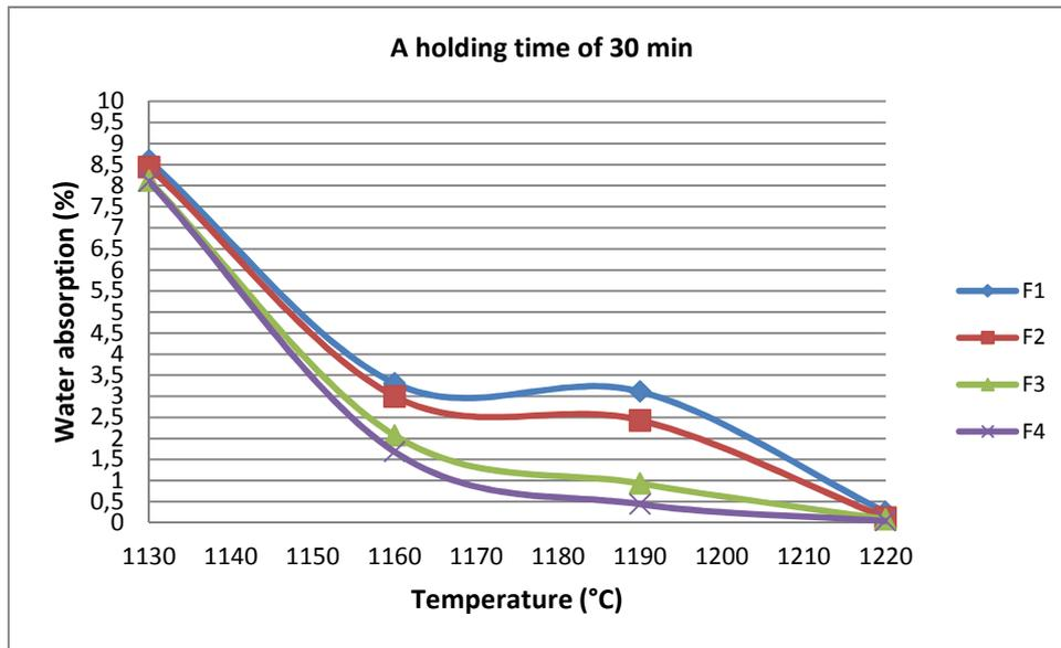
**Fig. 5. Water absorption (%) of the four formulas according to the temperature at holding time equal to 30 min**
