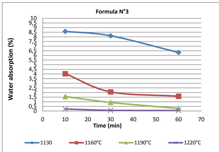
Fig. 3. Evolution of the water absorption of the formula n°3 according to the holding time at various temperatures of firing
