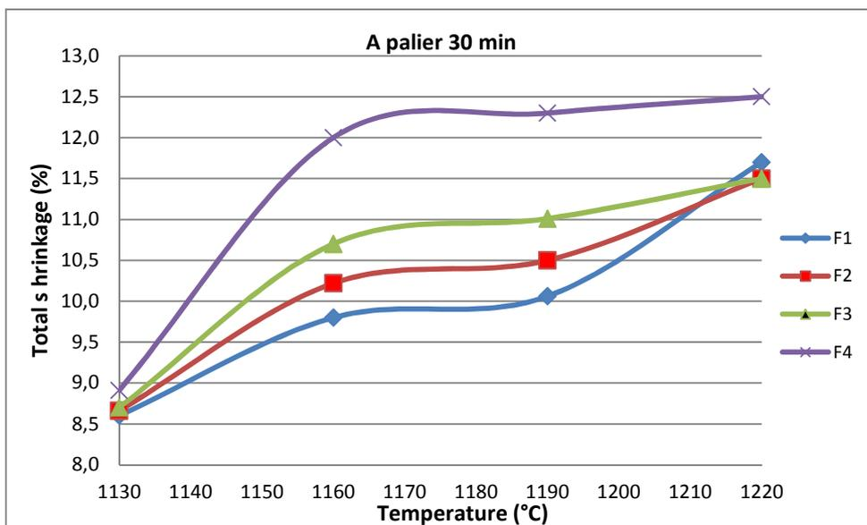
Fig. 6. The evolution of total shrinkage (%) of the four formulas according to the temperature at holding time equal to 30 min
