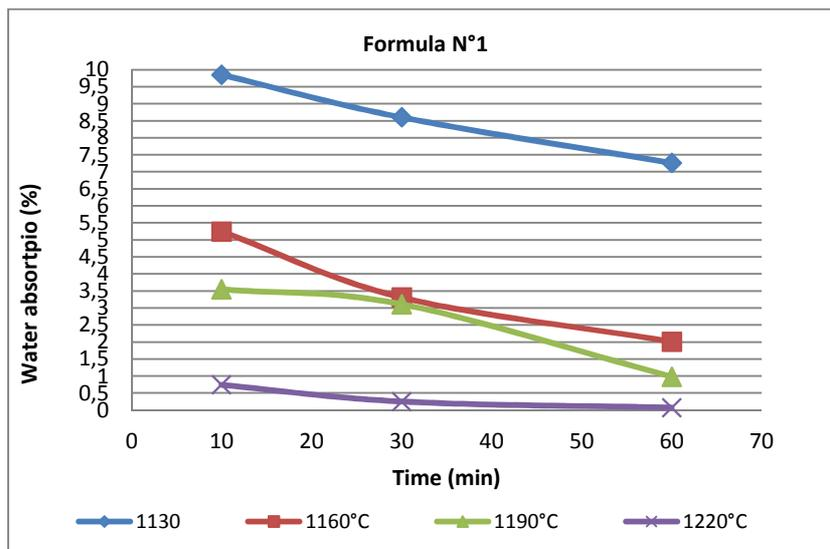
Fig. 1. Evolution of the water absorption of the formula n°1 according to the holding time at various temperatures of firing
