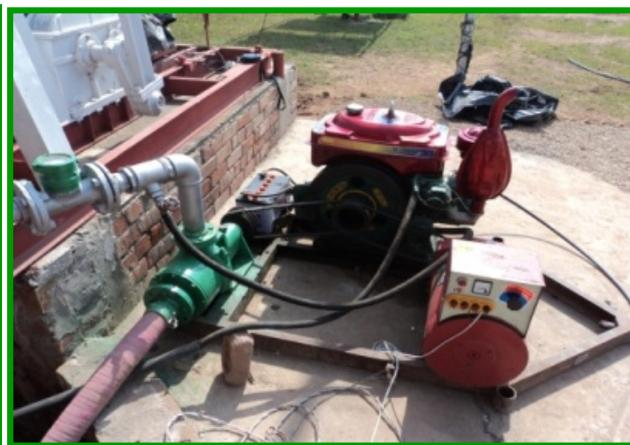
*Fig. 2 Dual-fuel Pumping system Installed at NARC, Pakistan*
