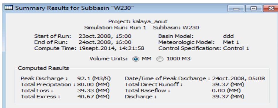
**Fig. 11.** Data derived from the Simulation of the hydrologic model
