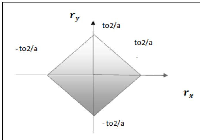
Fig. 6. Representation of the Deviations Domain E2B of perpendicularity
