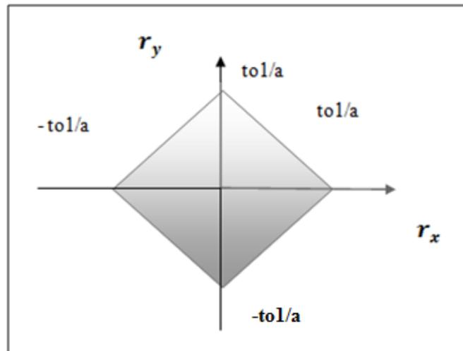
Fig. 5. Representation of the Deviations Domain E1B of perpendicularity
