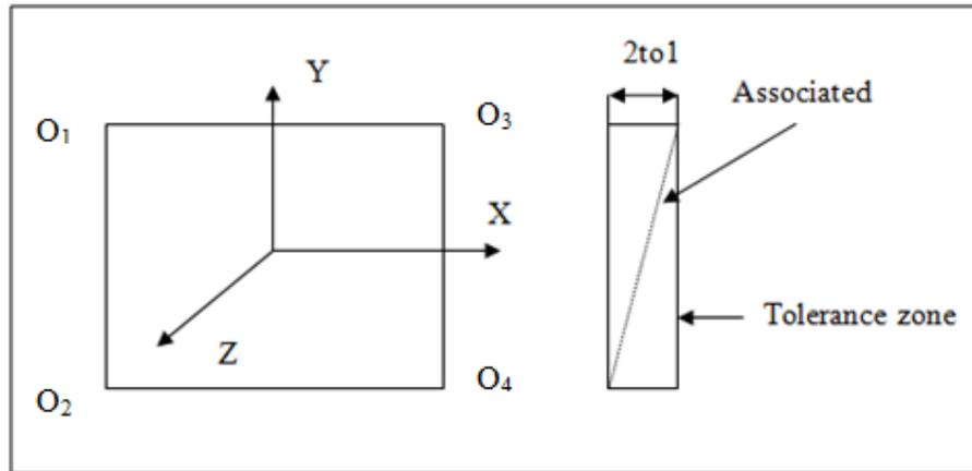
Fig. 4. Presentation of the tolerance zone of perpendicularity
