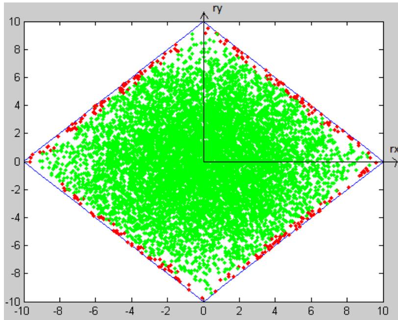
**Fig. 10. Statistical Tolerancing taking into account the form deviations**
