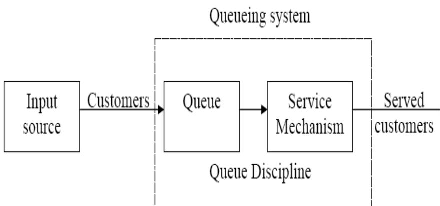
Figure 1: Characteristics Of Queuing System
