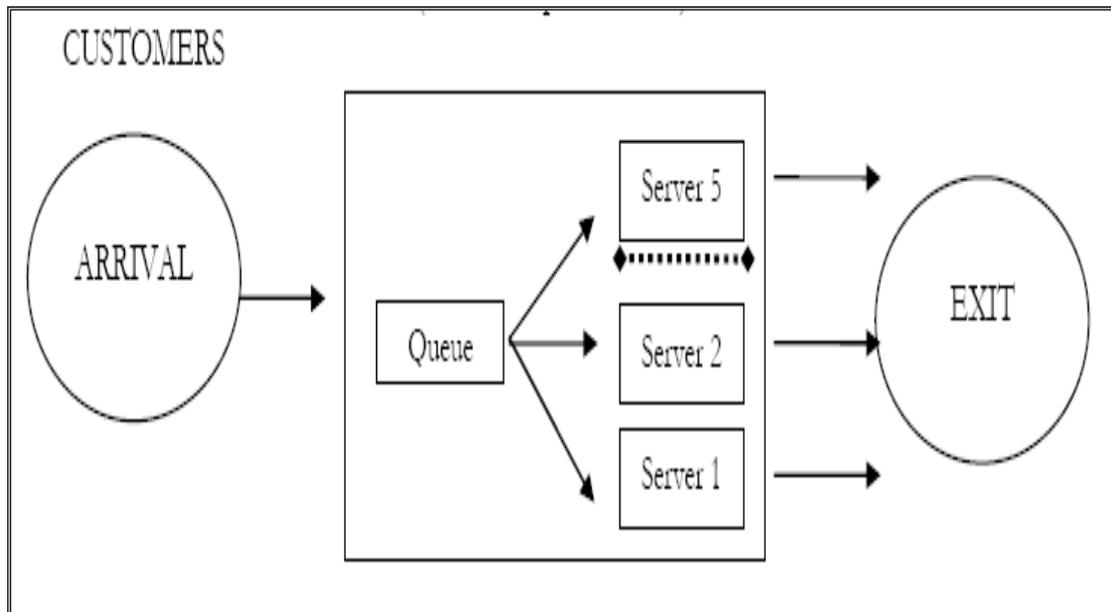
Figure 3: Single Queuing Model With Single –Queue And Multiple Parallel Servers
