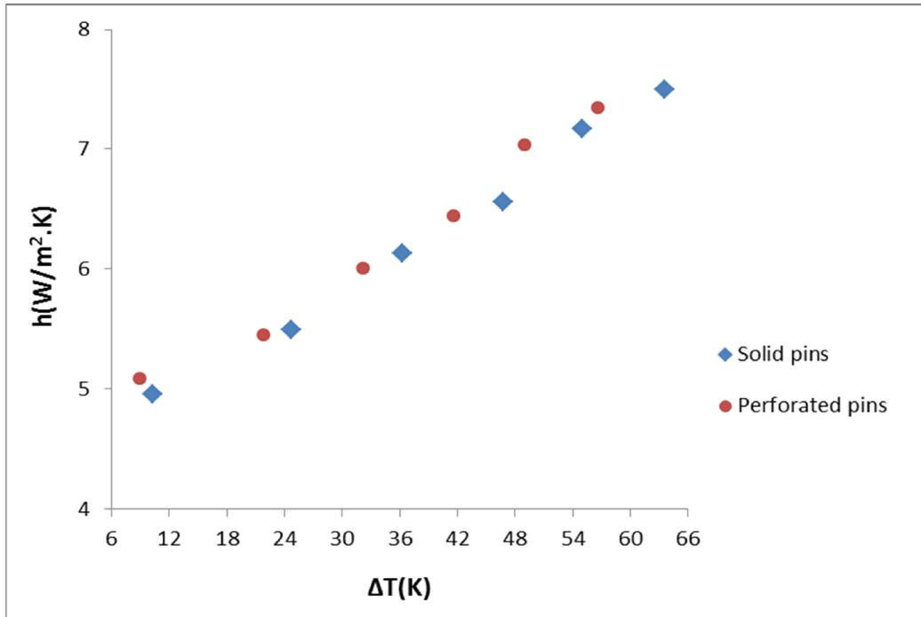
Fig. 3. Temperature difference variations  $\Delta T$  with average heat transfer coefficient  $h$  for solid and perforated heat sink
