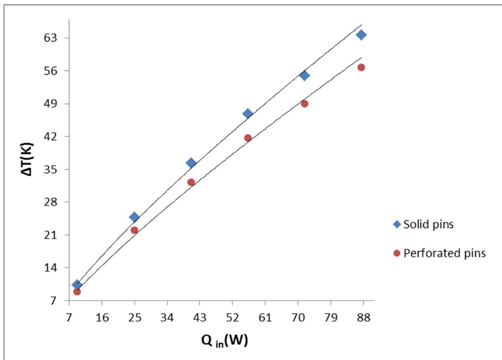
Fig. 2. Temperature difference variations  $\Delta T$  with heat input rate,  $Q_{in}$  for solid and perforated heat sink
