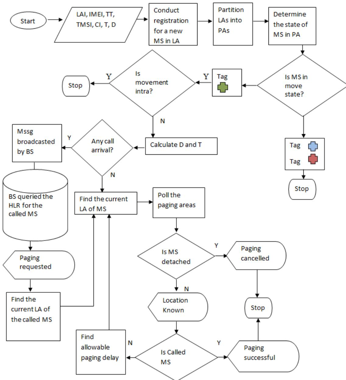
Figure 2: MSIP-GSM PROCESS FLOW
