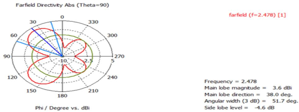
Fig. 10. Simulated radiation patterns in dB ( $\theta = 90$ , x-y plane) at fr=2.478 GHz
