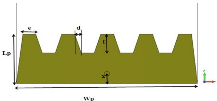
Fig. 2. the geometry of the top radiating plate
