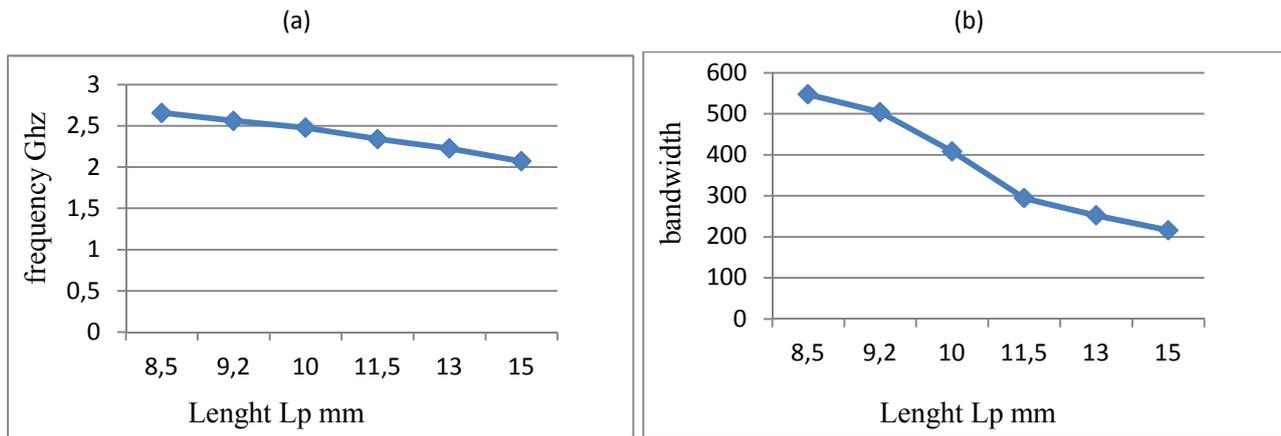
Fig. 5. Changes of length of the radiating plate according resonance frequency and bandwidth
