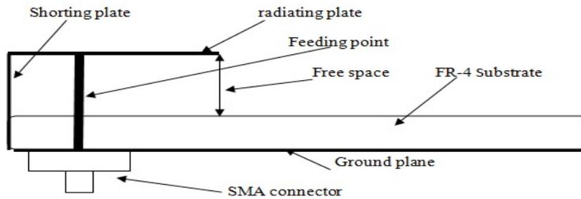
**Fig. 1. the geometry of the PIFA antenna proposed**
