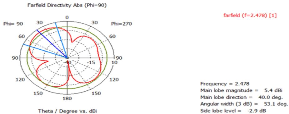
Fig. 9. Simulated radiation patterns in dB ( $\varphi = 90$ , y-z plane) at fr=2.478 GHz
