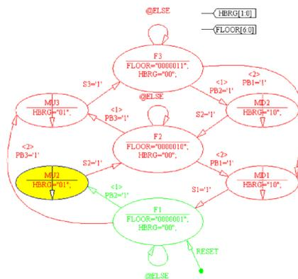
Fig. 3. Diagram for transition between floors
