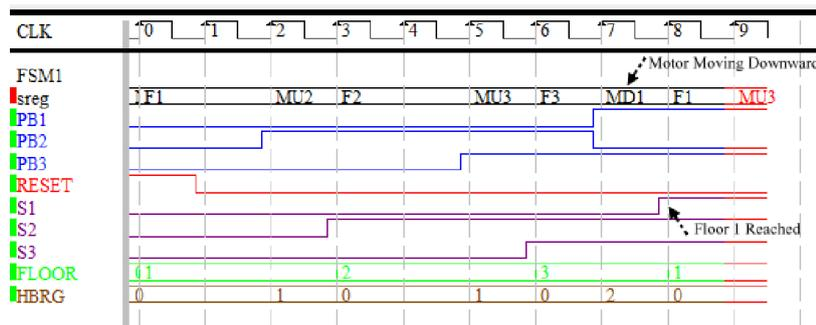
Fig. 8. Elevator moving downward for floor 1
