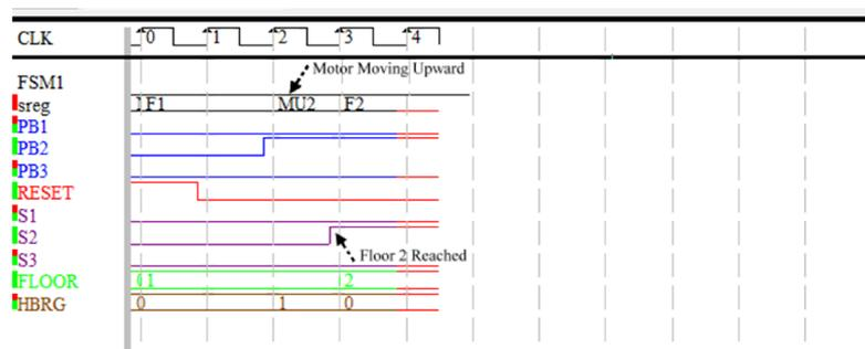
Fig. 6. Elevator moving upward for floor 2
