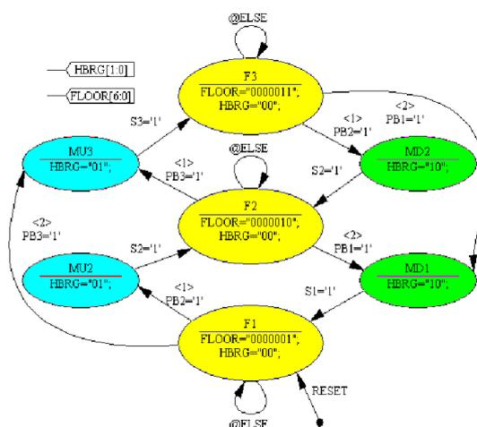
Fig. 1. Elevator control system
