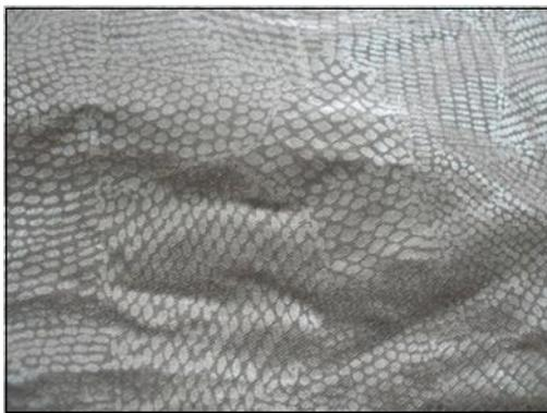
**Fig.16. Metallic cotton fabric/foil printed fabric**
