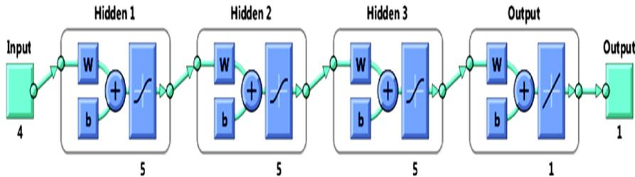
Fig. 7. Utilized Neural Network with 3 hidden layers
