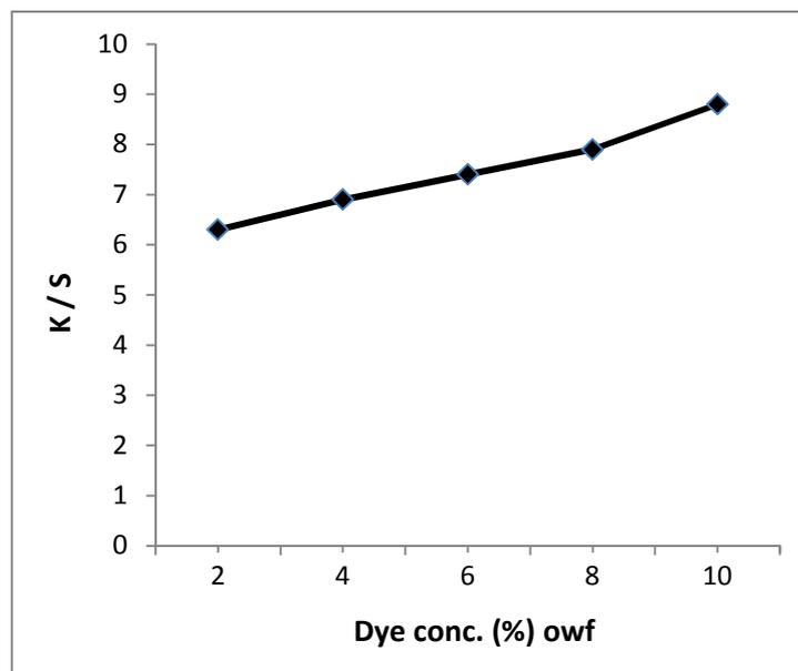
**Fig. 4.** Effect of Brazilwood natural dye conc. on the color strength (K/S) of dyed cotton fabrics
