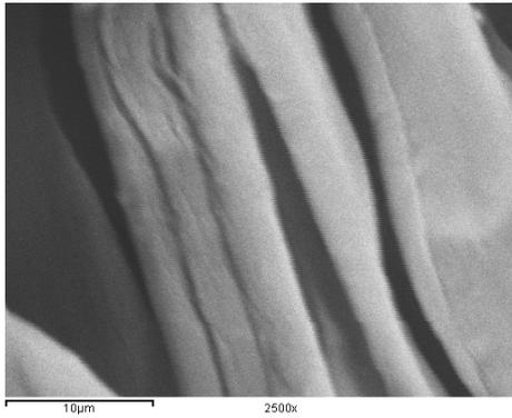
**Figure (12a): untreated cotton sample**
