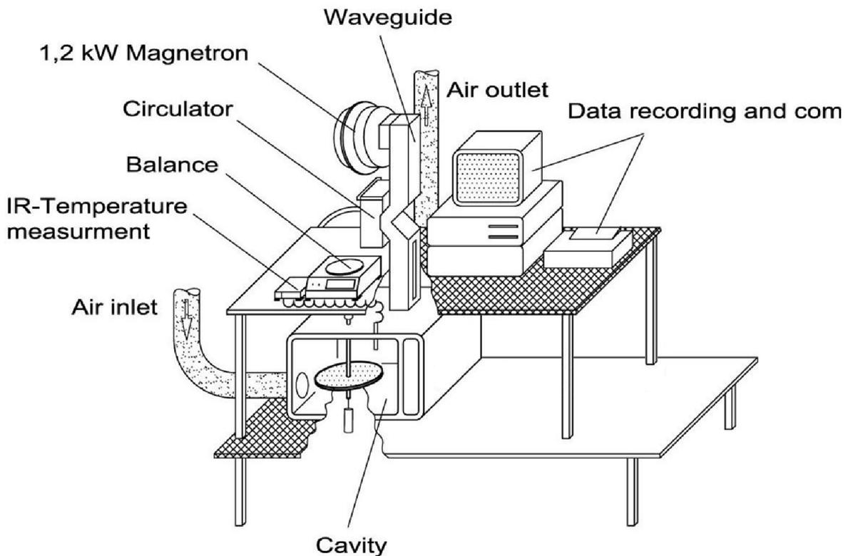
*Fig.1. Schematic diagram of the laboratory microwave system*
