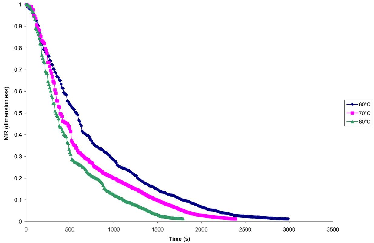
Fig. 4. Drying curves of moisture ratio versus drying time for the three temperatures
