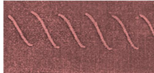
**Figure 6:**  $V_{A3}$  signal at the output of the inverter-follower (5V/div. - 5ms/div.)
