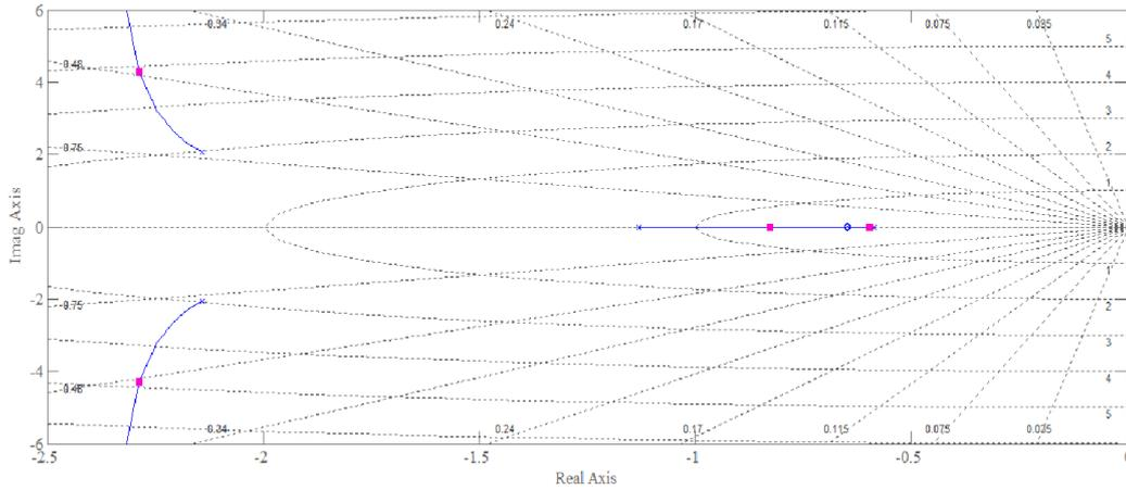
Fig.8. Root –locus diagram of the system by keeping, Kp=18
