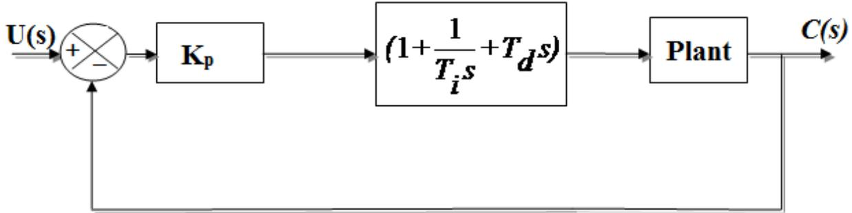
**Fig.2. Block diagram of Continuous PID Controller**
