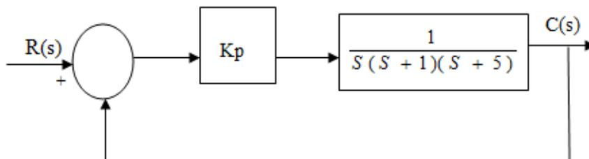
**Fig.3. Block Diagram of Controller and Plant**
