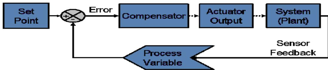
*Fig.1. Block diagram of a typical closed loop system*
