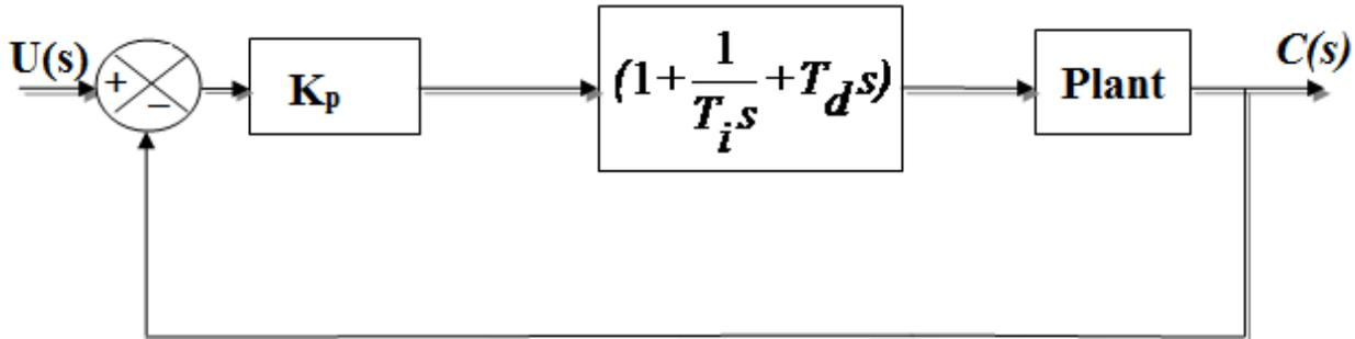
**Fig.2. Block diagram of Continuous PID Controller**
