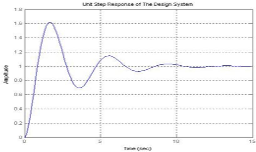
**Fig.6. Unit Step Response of the Designed System**
