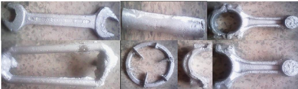
**Plate 3: Cast component after surface finishing**
