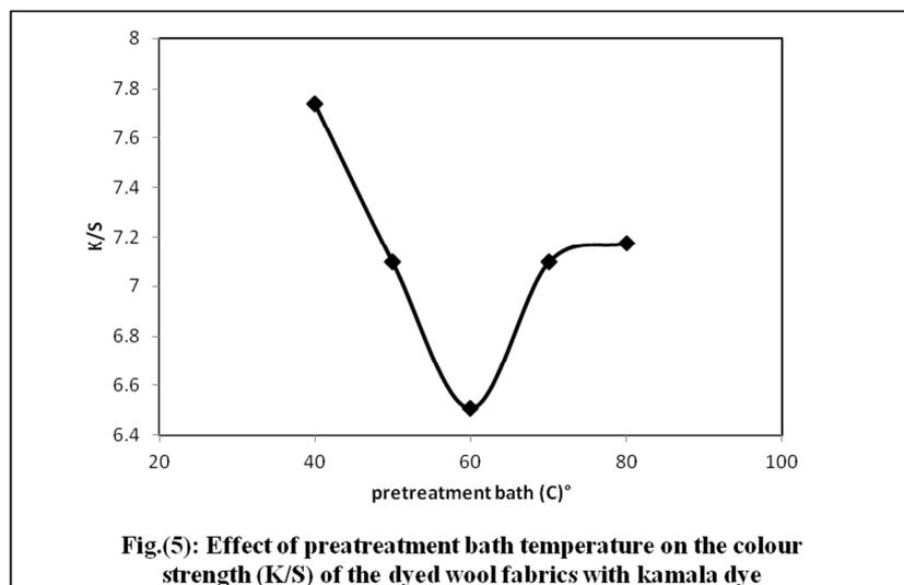
The results indicate that the most suitable temperature which establishes the maximum efficiency of the enzymes is at 40°C. This result because the enzyme is very sensitive to higher temperatures. The gap in hydrolytic activity was bigger depending on pH levels than on temperature values. [7]
