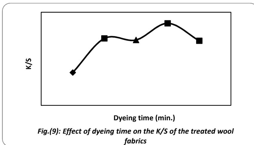
From the above figure, we can conclude that maximum K/S can be achieved when dyeing for 60 minutes at 80 °C. There will be a decrease when continue dyeing for longer than 60 min. and this may be attributed to the non stability of the dye molecules at long durations getting out from the fabric leading to that decrease in the K/S. Hence, it is preferable to dye at 80°C for one hour.
