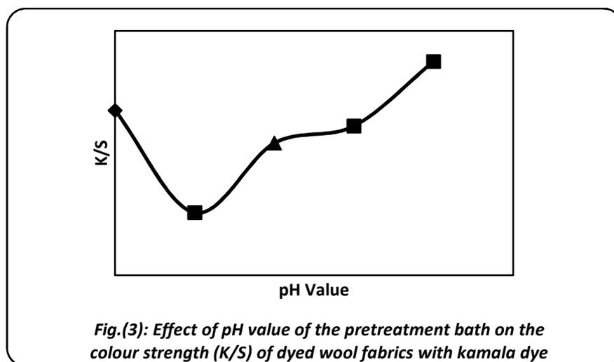
From the figure, it can be concluded that the best pH value of the treatment bath to achieve the most efficient enzyme performance is at pH= 8 and pH= 4 .The activity of an enzyme strongly depends on the pH and temperature. Below the optimum pH and temperature, the enzyme, a protein, is denatured or inactivated, which decreases enzyme activity.[7]
