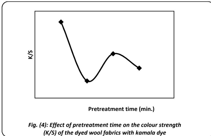
It is obvious from the former figure that performing the pretreatment process for 30 minutes gives the maximum colour strength. It is evident from the figure that lasting the time of pretreatment ends in decreasing of the K/S obtained. This may leads to a decreasing in the activity of the mixed enzymes in the extracted solution.
