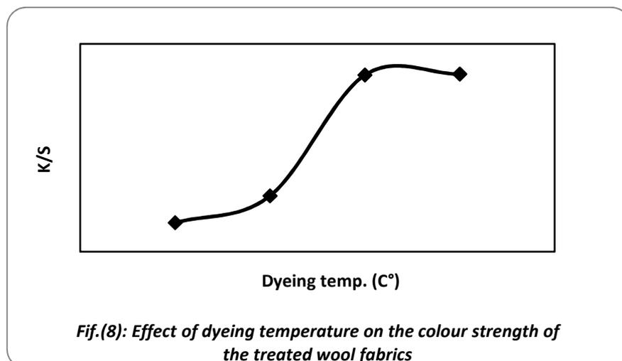
We can notice from the previous figure that the K/S value of the treated wool fabrics dyed with kamala was increased by increasing the dyeing temperature until reaching its highest value at 100°C. Although, the dyeing process can be applied at 80°C because no much difference between K/S values at these two points.
