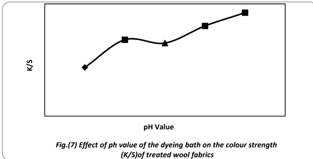
From the prior figure, we can conclude that maximum K/S was recognized at pH=8 and this may be attributed to the nature of the dye, which is insoluble in water and became dispersed by adding alkali. The higher the pH value, the higher the amount of alkali added to the bath. Hence the more soluble is the dye.
