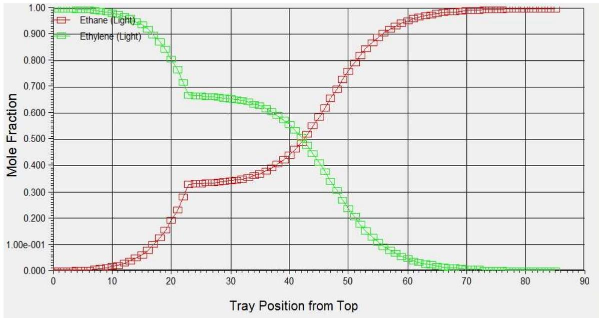
Figure 7: Mole fraction vs tray position from top
