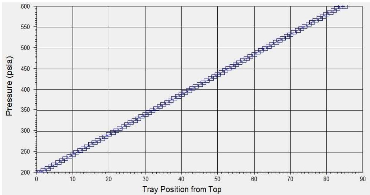
Figure 6: Pressure vs tray position from top
