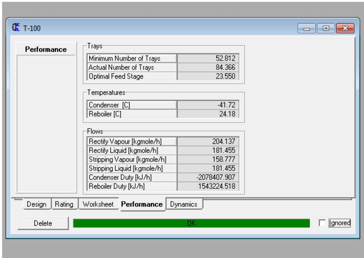
Figure 2: Performance of shortcut distillation column
