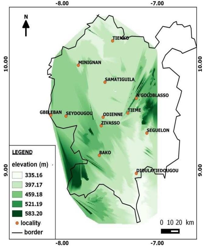
Figure4: DEM built with TIN interpolation method
