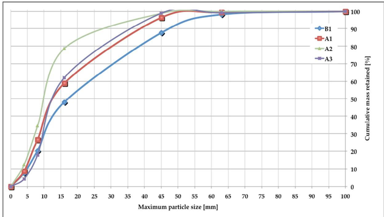
Fig. 1. Cumulative particles size distribution of test materials
