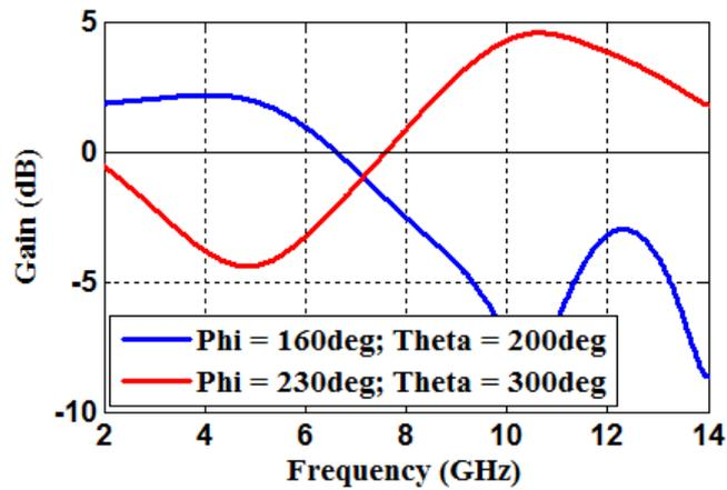
Fig. 8. Simulated gain of the proposed UWB antenna
