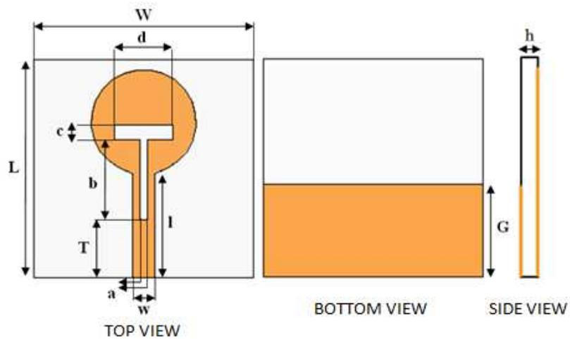
*Fig. 1. The geometry of the proposed UWB antenna*
