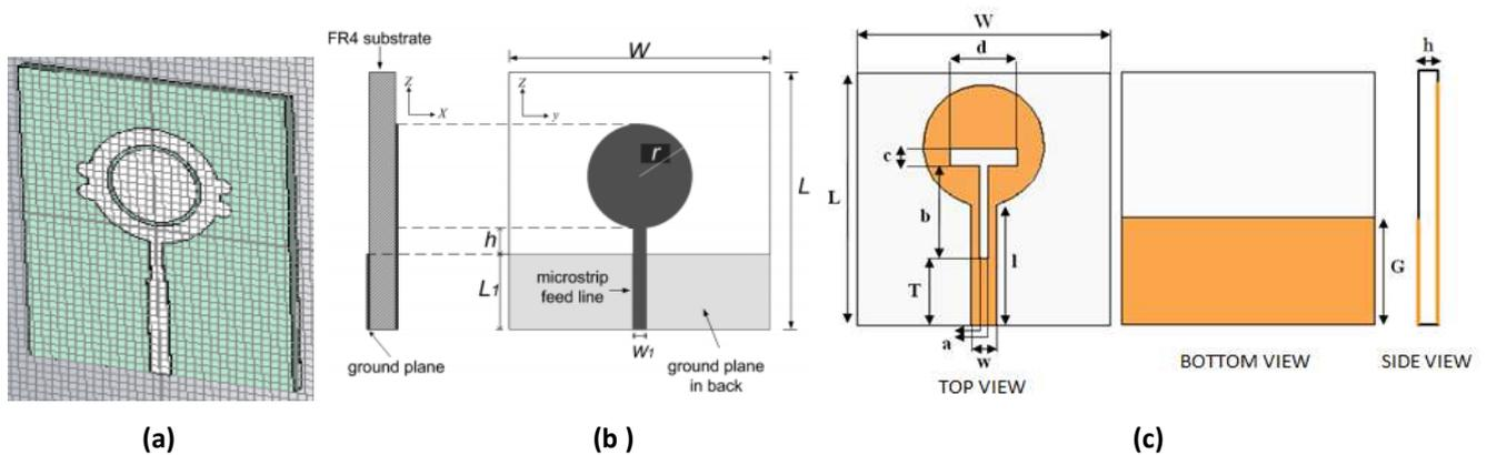
Fig. 10. Geometry of the reference antennas and the proposed antenna, (a) [11], (b) [12] and (c) proposed antenna
