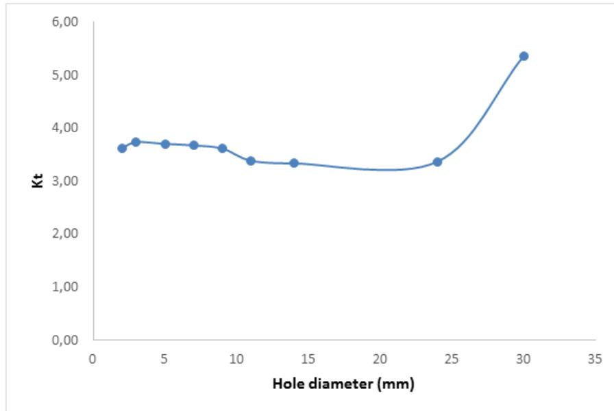
Fig. 6. Evolution of concentration coefficient of stress according to the size of the defect
