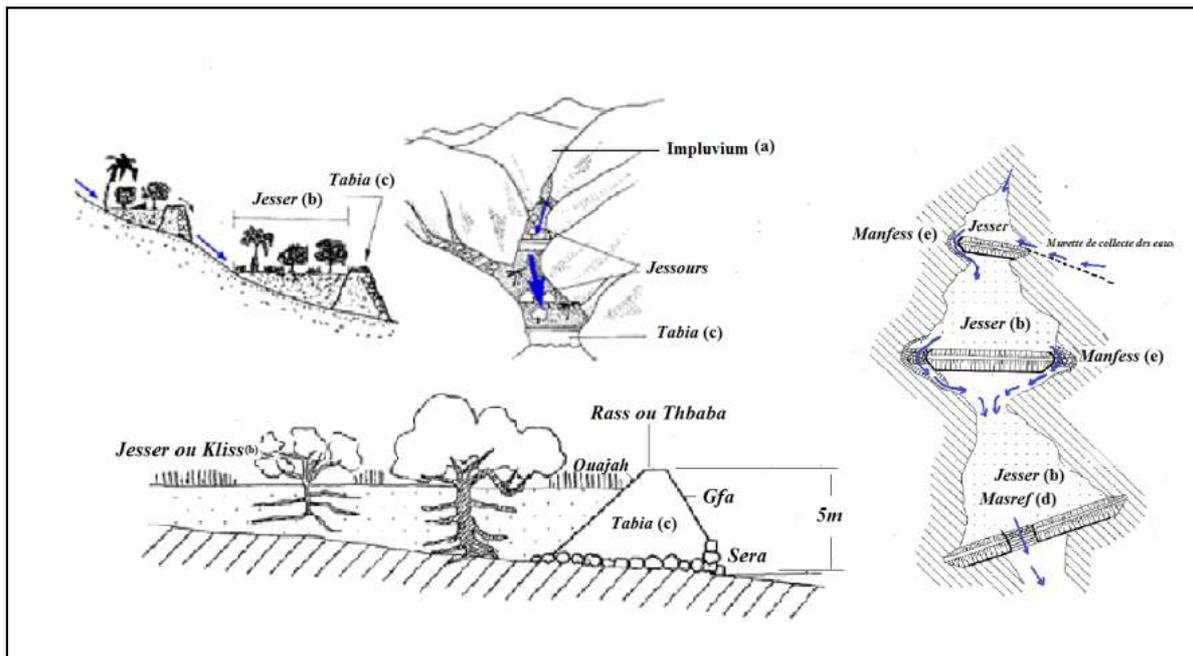
Fig. 1. Different components of the Jessours system (Adapted)
