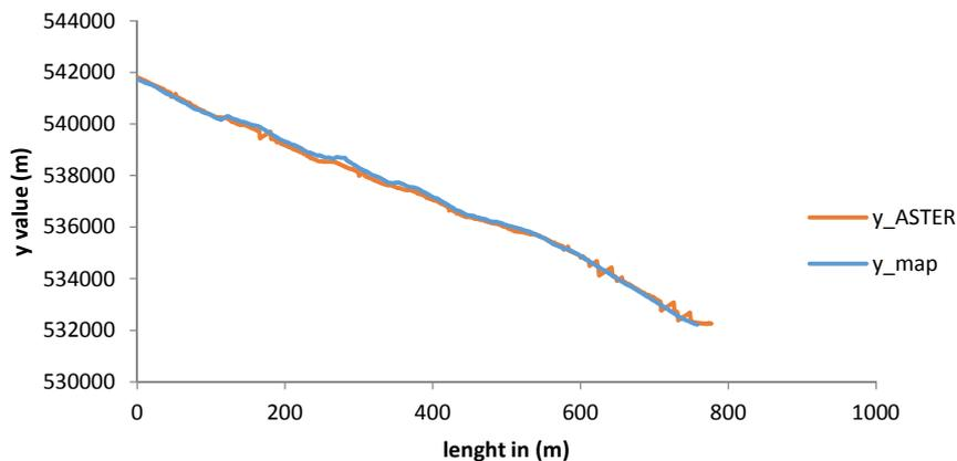
Figure 10. Y coordinates profile from the two drainage network along a river
