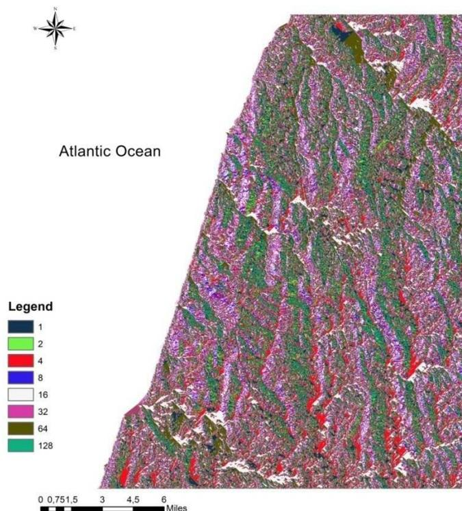
Figure 6. Flow direction map from ASTER DEM
