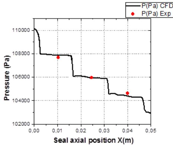
Fig. 8. Pressure distribution in the axial direction of the seal
