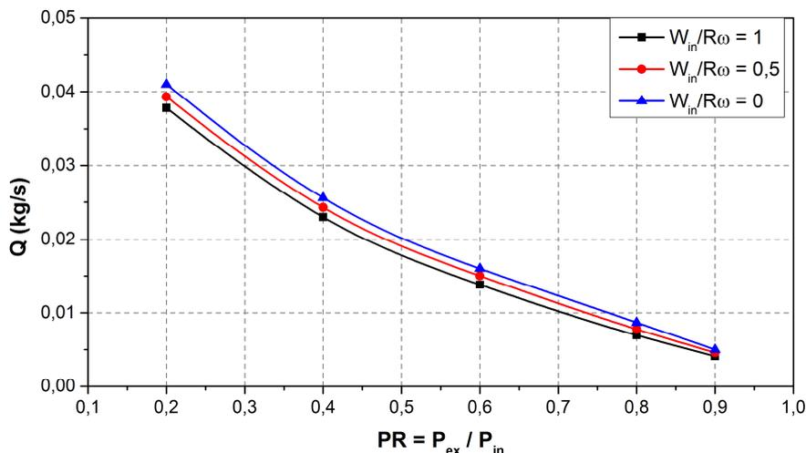
Fig. 12. Leakage flow versus pressure ratio with the non-dimensional inlet swirl as a parameter
