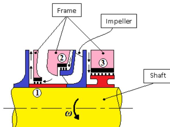
Fig. 1. Labyrinth seal sites in a compressor
