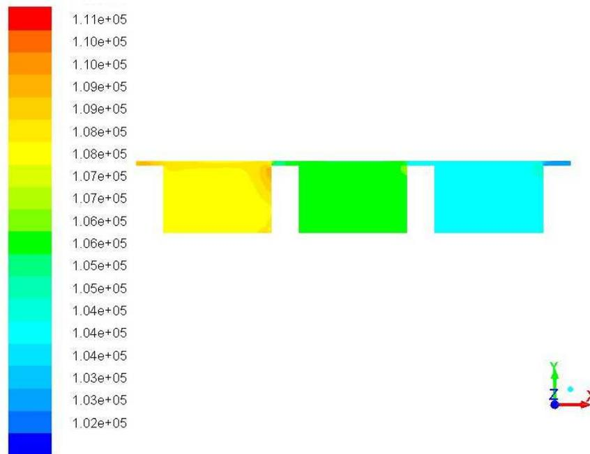
Fig. 9. Pressure contours in the XY plane of the seal
