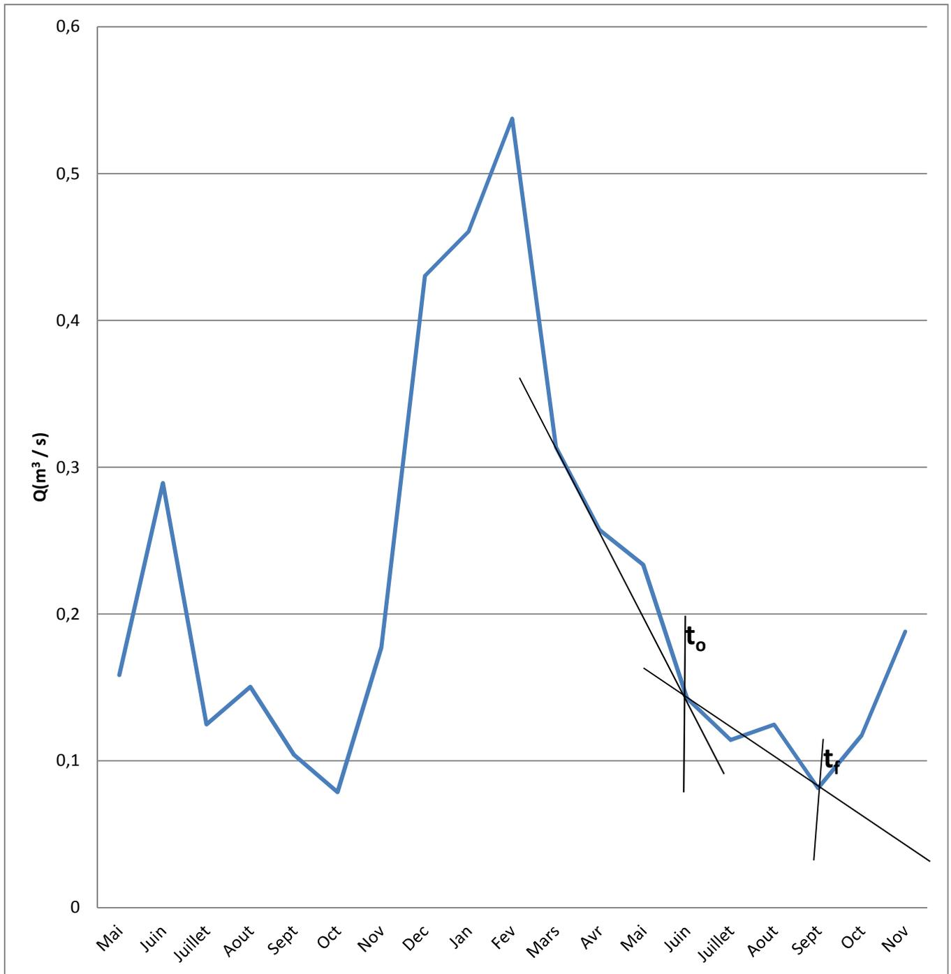
Fig. 3. Hydrogram of flood of Kisanga II (2014)
