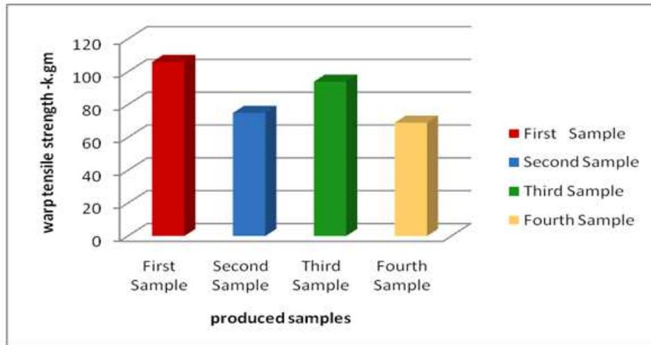
*Fig. 17. Effect of production method variation on tensile strength in warp direction*
