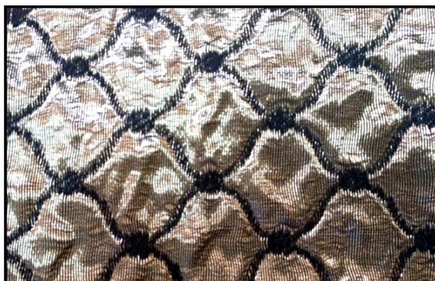
Fig. 9. The third sample which produced by weft waded double cloth method
