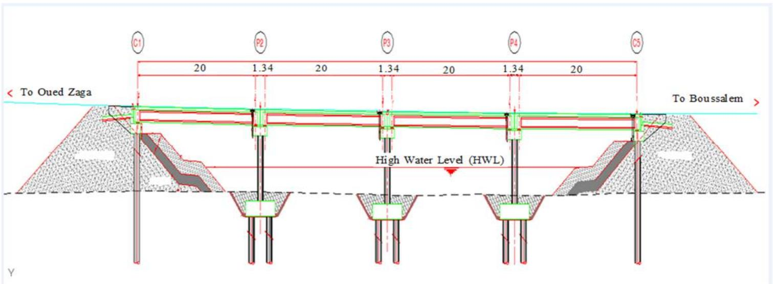
*Figure 2: Longitudinal section of the bridge*
