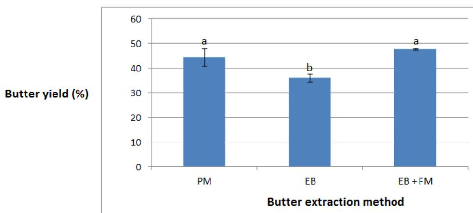
**Fig.5: Variation of yields according to artisanal extraction methods. PM = method by mechanical press, EB = traditional method using boiled water and EB + FM = traditional method using boiled water plus mango leaves.**
