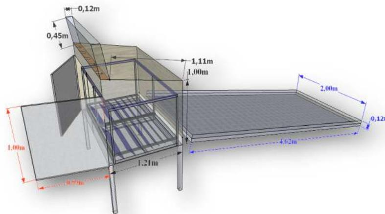
Fig. 2. Schematic of the experimental drying equipment [22]
