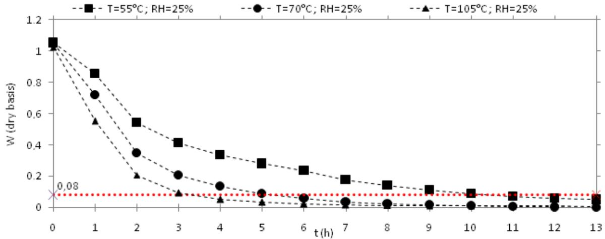
Fig. 4. Cocoa beans Moisture contents rate curves for 3 different temperatures.
