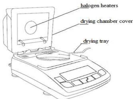
Fig. 1. Schematic diagram of the artificial drying equipment
