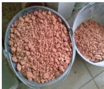
*Fig. 7. Clay-based artificial gravels 8/16 fired at 1100°C*
