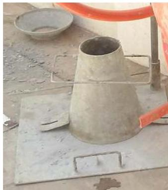
*Fig. 2. Slump test cone*
