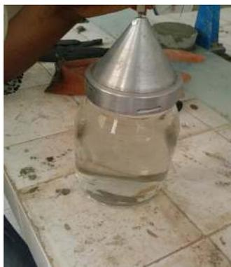
Fig. 10. Pycnometer filled with water
