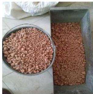
*Fig. 6. Clay-based artificial gravels 8/16 fired at 860°C*
