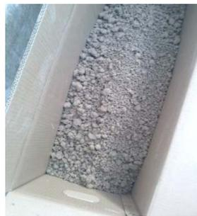
*Fig.5. Clay aggregates*
