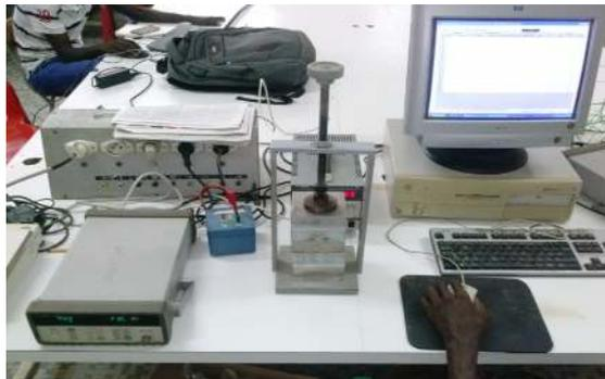
*Figure 19: Apparatus of the hot asymmetric plan method*
