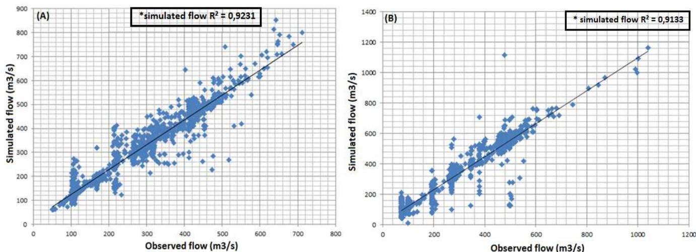
Fig. 7. Simulated versus observed flow, 5 years for calibration (A) and 3 years for validation (B)
