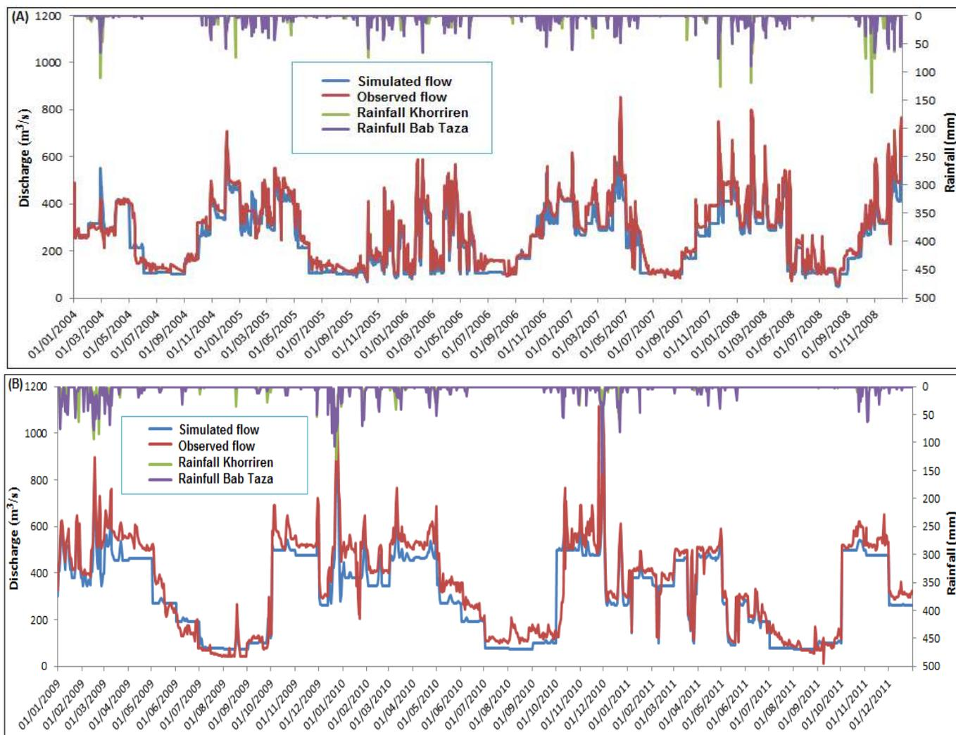
Fig. 6. Daily hydrograph comparison between simulated and observed flow for the catchments of Laou basin. A) Calibration period 2004-2008, B) Validation period (2009-2012).
