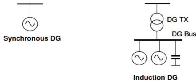
Synchronous distributed generation has the ability to remain stable even when a grid faults [3]. This ability is attributed to the stability of rotor angle. The rotor angle stability is determined using the critical area method or what is commonly known as the equal area criterion [3]. Synchronous distributed generation affects voltage stability thereby making a matter of interest for this paper and particularly this chapter.
