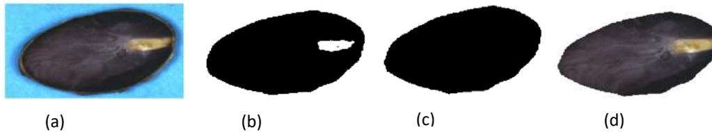
Fig. 4. Segmentation process: (a) Original image, (b) Otsu's thresholding, (c) Morphological opening, (d) segmented image
