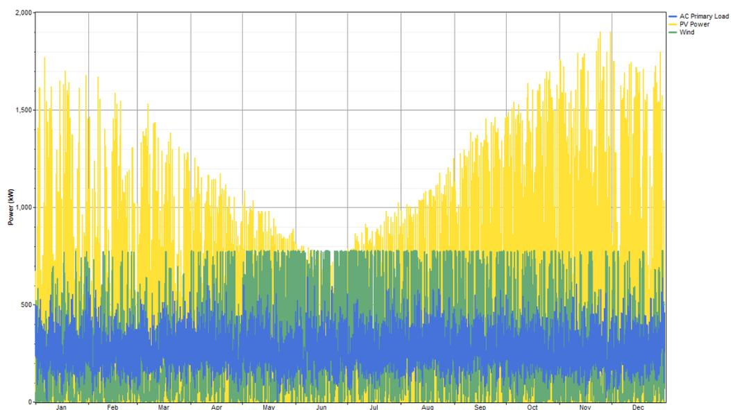
Fig. 13. Monthly evolution of the energy consumed by the load and produced by the wind turbines and by the PV field
