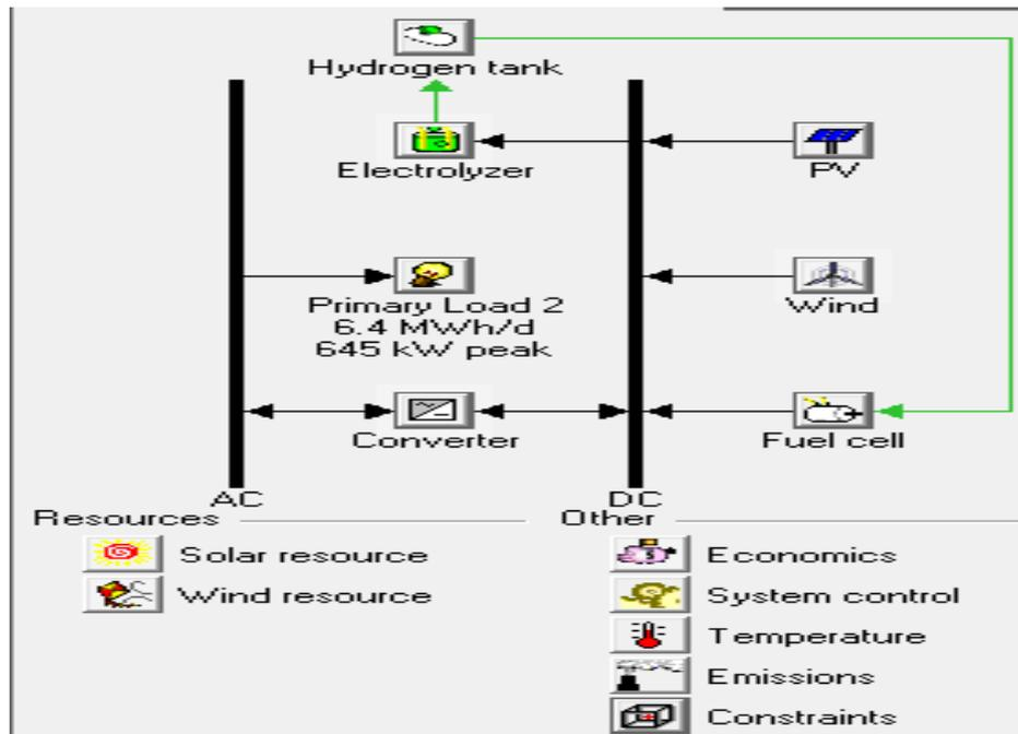
Fig. 1. Architecture of a micro-grid based on ENR system and hydrogen storage
